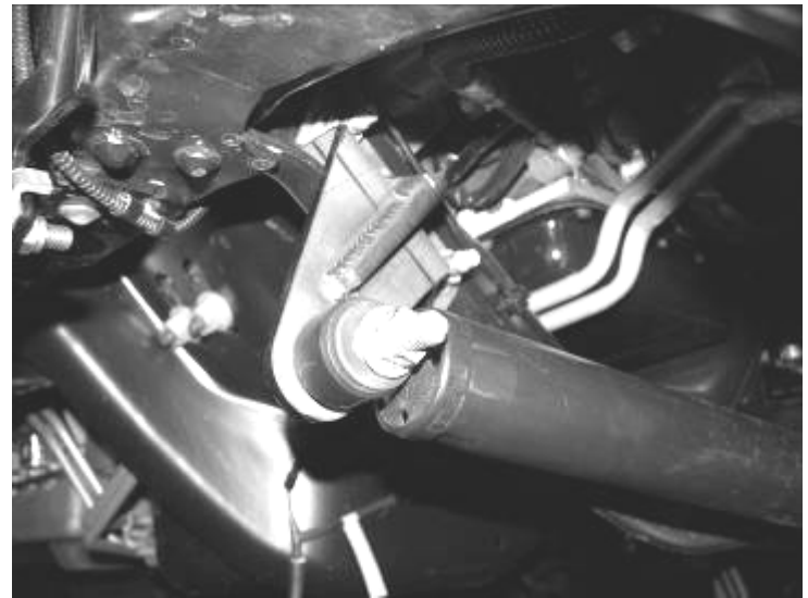
Picture Shown with Factory Stabilizer re-installed
