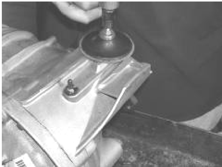
After Cut & Sanding Surface Smooth
