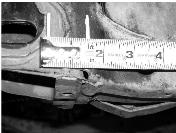
Measure 1 ½" inward from the cam pocket For cutting on both sides
