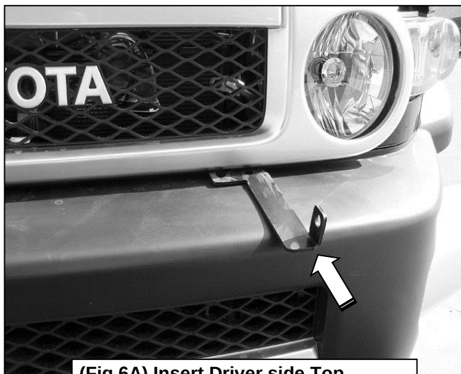
(Fig 6A) Insert Driver side Top Bracket through gap above bumper
