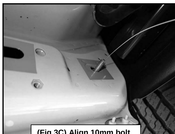
(Fig 3C) Align 10mm bolt in slot. Driver side shown
