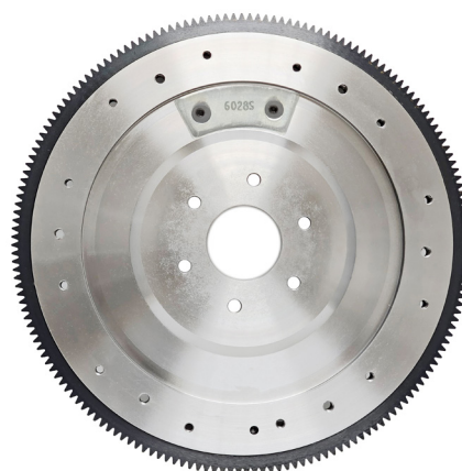
1646083 FOR 429-460BB EXTERNAL BALANCE 28 IN/OZ.W/6028S COUNTERWEIGHT
