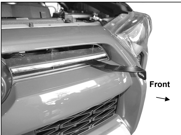
(Fig 14) 2014-on, driver/left Top Bracket installed
